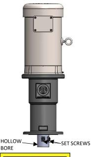
2.) ALIGN THE SHAFT POCKETS WITH THE SET SCREW HOLES IN THE HOLLOW BORE.
