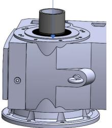
5.) POSITION THE SHAFT SO IT'S FLUSH WITH THE HOLLOW BORE OR AS INDICATED ON THE APPROVAL (OR AS MANUFACTURED) DRAWING.
