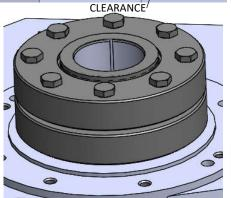
Size Size **Torque** Torque 64 in-lb. M5 8 62 in-lb. 110 in-lb. 10 106 in-lb. M6 13 22 ft-lb. 23 ft-lb. **M8** 46 ft-lb. 17 44 ft-lb. M<sub>10</sub> 77 ft-lb. M12 19 74 ft-lb. M16 24 184 ft-lb. 191 ft-lb. M20 30 361 ft-lb. 375 ft-lb. M24 36 620 ft-lb. 645 ft-lb. 46 1254 ft-lb. 1304 ft-lb. M30
