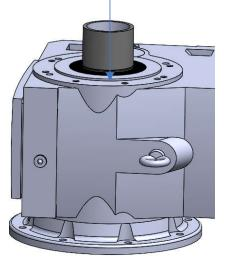
4.) IT'S IMPORTANT TO NOTE THAT IN SOME CASES THE GEARBOX HOLLOW BORE, TORQUE SIDE BUSHING, SHRINK DISK, AND SHAFT WILL BE MARKED WITH HAMMER PEENS AND PAINT PEN MARKS 90° APART. IF PRESENT, ENSURE THAT ALL OF THESE MARKS LINE UP.
