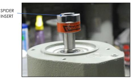
5) Once the drive coupling is in place mount the bearing housing using the appropriate bolts. Use lock washers or service removable thread locker on the bolt threads to prevent the bolts from vibrating loose. Ensure that the couplings are properly engaged without any excess pressure against the spider. Excessive vibration may occur at start up if the hubs are pressed too tightly together causing excess pressure against the spider which will also causes excess axial pressure against the bearings.
