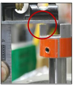
Note the 1/16" gap between square's arm and coupling tooth. A penny can be used to set this spacing.
