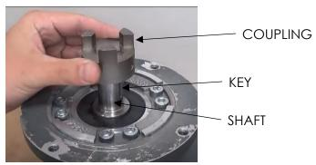
3) Based on the coupling size, use the table to select the appropriate subtract distance "X". Subtract this value from the measured distance from step 1 to get the coupling placement distance.
