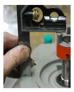
5) Tighten the set screw(s) to the appropriate value from the table below. Place the spider insert into the motor's coupling.
