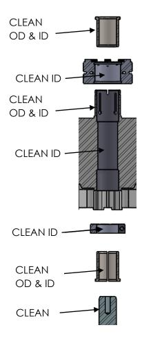
3) Position the clamp ring and lower bushing over the machine shaft as shown below. Make sure the bushing and clamp are in its desired location. The end of the shaft should be flush with the top of the upper bushing as shown on page 1. Once the position is verified, secure the support bushing with the clamp ring and tighten the clamp ring screw.
