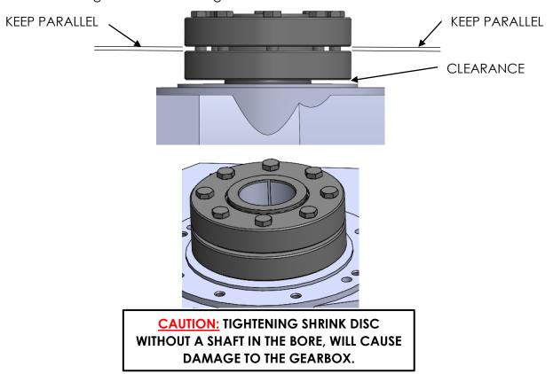
7) Tighten the bolts in a circular pattern using 1/4 (90°) turns, even if some bolts initially require very low tightening torque to achieve 1/4 turns. ENSURE THE SHRINK DISC IS TIGHTENING EVENLY AND PARALLEL. Tighten to the appropriate "tightening torque" value in the table on next page.
