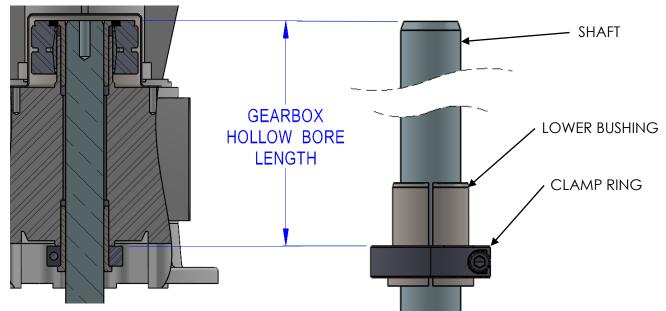
4) Without taking the shrink disc apart, verify all the bolts on the shrink disc are loose and slide the shrink disc onto the hollow bore OD. Slide the upper bushing into the gearbox hollow bore. The gearbox is now ready for the shaft installation.
