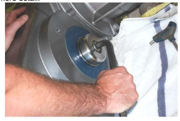
4. Pre-Lubrication: Make sure that all grease fittings are lubricated on the motor, gearbox, and pedestal. On larger units, the input bearing on the gearbox comes with an automatic lubricator, which needs to be activated before use. See the
