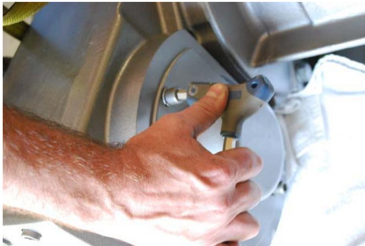
Remove the dust cover off of the back of the gearbox. It would be best to lock the shaft in position with a non galling wrench or collar.
