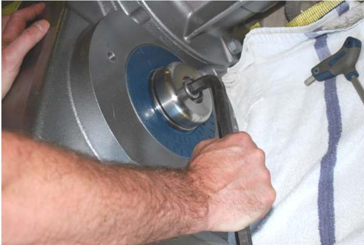
Remove the cap plate from the gearbox. You may need to lock the shaft from rotating with a non-galling wrench.
