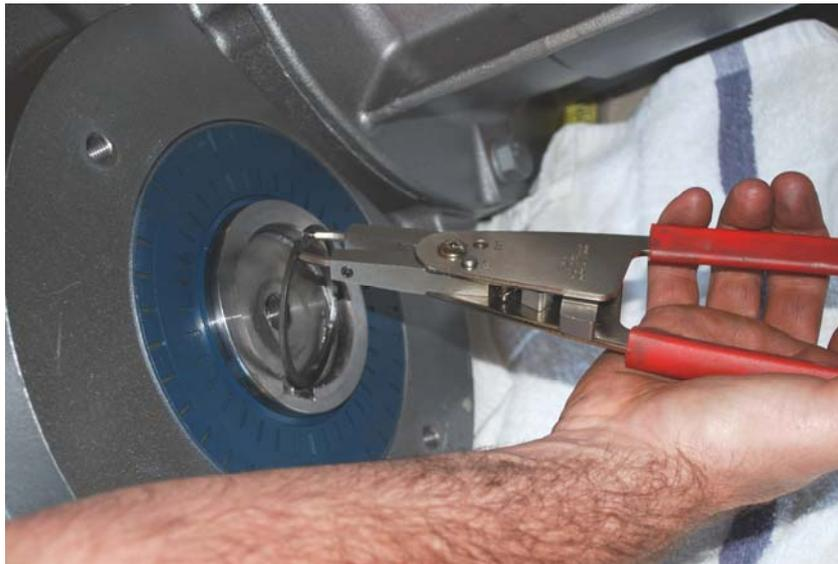
Remove the snap ring from the hollow bore.
