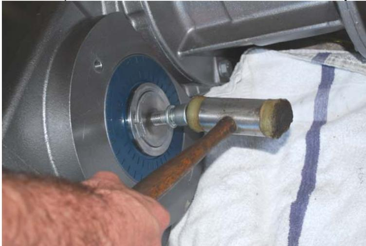
This will allow you to tap the shaft back into place with a plastic mallet to re-install the snap ring and cap plate. **THE SNAP RING MUST GO BACK INTO PLACE!!!** Once the snap ring and cap plate are back in place, torque cap plate to ~half the full torque value of the bolt and install the dust cover. See below:
