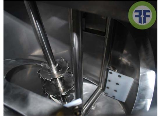
**DUAL SHAFT SANITARY MIXING SYSTEM - INTERIOR**
