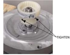
6.) MOUNT THE MOTOR ONTO THE GEARBOX INPUT ADAPTER WITH THE APPROPRIATE BOLTS, USE LOCK WASHERS OR SERVICE REMOVABLE THREAD LOCKER TO PROHIBIT BOLTS FROM VIBRATING LOOSE. ENSURE THAT THE COUPLINGS ENGAGE SECURELY.
