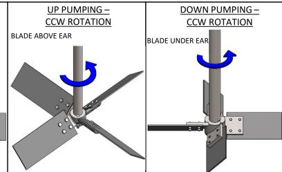
DAMAGE IS HIGHLY LIKELY IF THE BLADES ARE MOUNTED ON THE WRONG SIDE OF THE HUB'S EARS OR ROTATION IS INCORRECT.
