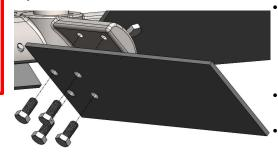
BLUE 242 LOCTITE OR SIMILAR SERVICE REMOVABLE THREAD-LOCKER RECOMMENDED. CHECK PROCESS
