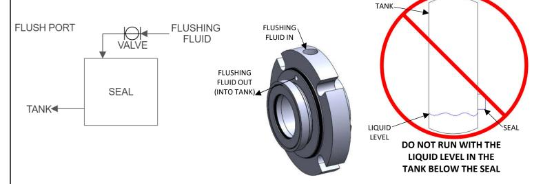
IF FLUSH PORT ISN'T BEING USED IN OPERATION OR FOR CLEANING, INSTALL A PLUG. **LEAVING THE FLUSH PORT OPEN WILL RESULT IN LEAKING.**
