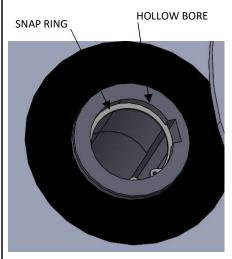
3.) INSERT THE KEY INTO THE KEYWAY OF THE SHAFT. DEBURR, CLEAN, THEN LIGHTLY LUBRICATE THE SECTION OF THE SHAFT THAT WILL GO INTO THE
