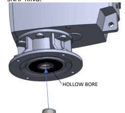
5.) ATTACH THE SHAFT TO THE GEARBOX USING THE FIXING ELEMENT AND FIXING ELEMENT BOLT (BOTH PROVIDED). APPLY SERVICE REMOVABLE THREAD LOCKER TO THE BOLT AND TIGHTEN TO THE APPROPRIATE VALUE IN THE TABLE.
