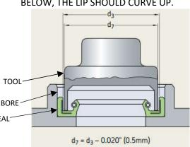
B.) REMOVE THE LIP SEAL(S) FROM THE PEDESTAL BORE BY EITHER TAPPING THEM OUT FROM THE BOTTOM OF THE PEDESTAL OR PRY THEM OUT FROM THE PEDESTAL WINDOW.
