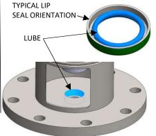
F.) USE A SHORTER PIECE OF WOOD AND THIS PATTERN TO DRIVE THE SEAL FULLY INTO THE BORE.
