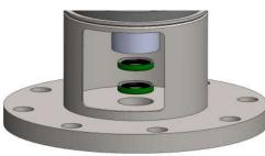
E.) IF YOU ARE UNABLE TO GET OR MAKE A TOOL LIKE THE ONE ABOVE, USE A WOODEN BLOCK THAT'S LONG ENOUGH TO SPAN THE SEAL'S OUTSIDE DIAMETER AND A DEAD BLOW HAMMER. MAKE SURE TO TAP THE SEAL INTO THE BORE FOLLOWING THE PATTERN IN THE IMAGE TO AVOID TILTING OR SKEWING THE SEAL IN THE BORE.
