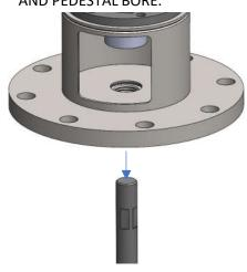
B.) USING SNAP RING PLIERS, REMOVE THE SNAP RING FROM THE GROOVE IN THE PEDESTAL. KEEP FOR RE-INSTALLATION.
