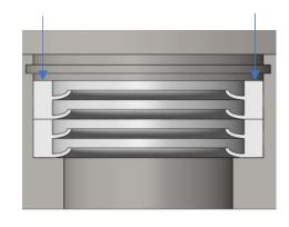
E.) RE-INSTALL THE SNAP RING WITH SNAP RING PLIERS, MAKING SURE IT'S FULLY SEATED IN THE SNAP RING GROOVE.
