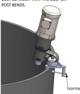
5.) LOOSEN THE 5/8" BOLT TO DIRECT THE BORE TOWARDS THE FOCAL POINT (REFER TO IMAGES ABOVE). ONCE THE **DESIRED LOCATION IS FOUND, TIGHTEN** THE 5/8" BOLT TO 92 FT-LB. INSTALL SHAFT AND IMPELLER(S) PER THE IMPELLER INSTALLATION QSG AND APPROPRIATE SHAFT INSTALLATION
