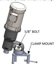
2.) LOOSEN THE LOWER CLAMP BOLT TO ALLOW FOR ENOUGH ROOM BETWEEN IT AND THE LOWER CLAMP PLATE PINS FOR THE MOUNT TO
