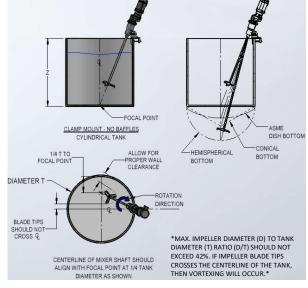
4.) TIGHTEN THE LOWER CLAMP BOLT SO THE MIXER IS STABLE AND SECURE TO THE TANK. DO NOT TIGHTEN THE **BOLT SO MUCH THAT THE BOLT OR**
