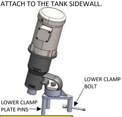
DISCONNECT MIXER FROM POWER SOURCE BEFORE ASSEMBLING, LIFTING, MOVING, OR SERVICING MIXER. 3.) REFER TO THE IMAGES BELOW FOR THE OPTIMAL MOUNTING POSITION. LIFT MIXER TO THIS POSITION AND SET THE CLAMP MOUNT ON THE TANK SIDEWALL.
