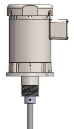
4.) WITH A 5/32 ALLEN, TIGHTEN THE FIRST SCREW UNTIL IT INITIALLY TOUCHES THE SHAFT. NOW, ROTATE THE SHAFT BACK AND FORTH WHILE TIGHTENING THE SCREW TO MAKE SURE IT'S ON THE DEEPEST PART OF THE FLAT. NOW TIGHTEN THE BOTTOM SET SCREW AND TIGHTEN BOTH SET SCREWS TO 103 IN-LB.
