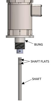
3.) INSERT SHAFT INTO SHAFT COUPLING, FLATS ON SHAFT SHOULD ALIGN WITH HOLES IN SHAFT COUPLING
