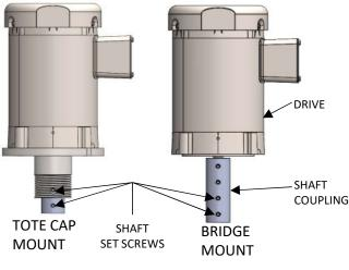
2.) ALIGN THE FLATS ON THE SHAFT WITH THE SET SCREW HOLES IN THE SHAFT COUPLING
