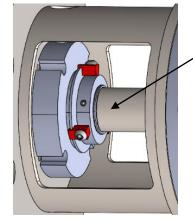
APPLY OIL OR GREASE TO SHAFT – THIS WILL HELP WITH THE NEXT STEP TO SLIDE SEAL ON SHAFT
