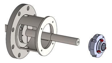
2-9) Reverse the seal removal steps to install a new or rebuilt seal. Follow the appropriate Seal Installation instructions for your application. Use Fusion Manual **FM-1033** for RT153 Seal Installation. Be careful to not cut O-ring on the new or rebuilt seal and use a process-compatible lubricant on the O-rings before installation.
