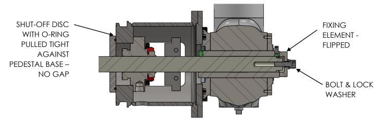
1-6) Flip the fixing element around so the side with the counterbore is facing towards the gearbox as shown below. This must be done so the shaft can be pulled into counterbore area. Insert the bolt & lock washer. Once bolt is engaged to the threads in the shaft, tighten to secure the shut-off.
