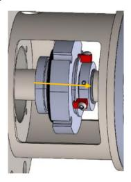
2-4) Install the shaft hold collar, in the orientation as shown below. The two shaft hold collar screws will have to be removed completely so the two shaft hold collar halves can be placed around the shaft. Reinstall the two shaft hold collar screws, leave them loose so the shaft collar can still slide on the shaft.
