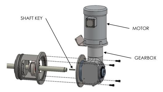
2-8) Slide the seal off the end of the shaft to remove. Follow appropriate instructions if the seal is to be rebuilt or replaced.
