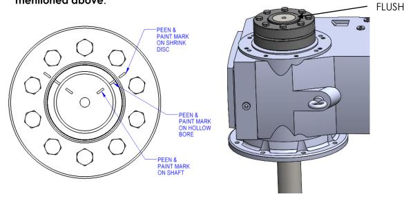
5) Verify there is clearance between the gearbox and the shrink disc. Hand tighten 3 or 4 equally spaced bolts. MAKE SURE THE OUTER COLLARS OF THE SHRINK DISC ARE DRAWN TOGETHER IN A PARALLEL FASHION. Then hand tighten the remaining bolts. DO NOT TIGHTEN THE SHRINK DISC WITHOUT A SHAFT IN THE BORE OF THE GEARBOX, AS THIS WILL CAUSE DAMAGE TO THE GEARBOX.
