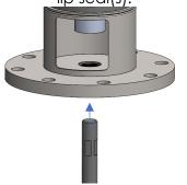
CHECK FOR SHARP EDGES OR **BURRS ON SHAFT BEFORE INSERTING** THROUGH LIP SEAL. DEBURR AS NECESSARY TO PREVENT CUTTING **OR TEARING LIP SEAL.**
