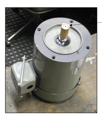
If replacing the motor & your motor has this style coupling, be sure to remove for use on the new motor.
