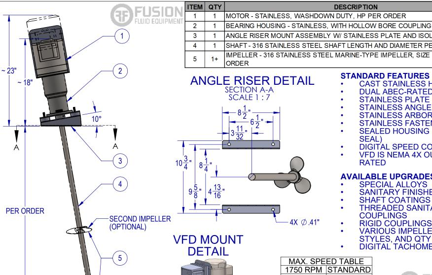
ANGLE RISER MOUNT ASSEMBLY W/ STAINLESS PLATE AND ISOLATION MOUNTS SHAFT - 316 STAINLESS STEEL SHAFT LENGTH AND DIAMETER PER ORDER IMPELLER - 316 STAINLESS STEEL MARINE-TYPE IMPELLER, SIZE AND QTY PER
