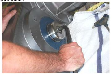
4. Pre-Lubrication: Make sure that all grease fittings are lubricated on the motor, gearbox, and pedestal. On stuffing box units, <u>be sure to lubricate the packing gland lantern ring with process compatible grease</u>. On larger units, the input bearing on the gearbox comes with an automatic lubricator, which needs to be activated before use. See the figures below for more detail:
